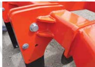
Replacable shear bolts
